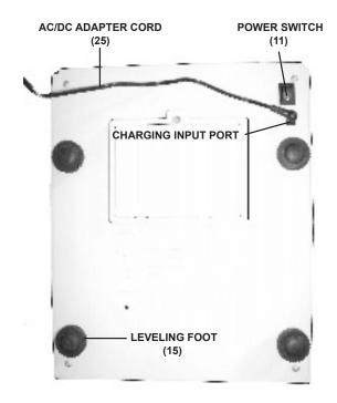
To charge the Battery (21) of the Scale, insert the AC/DC Adapter (25) Cord into the Charging Input Port located on the underside of the Scale. Make sure the Power Switch (11) is in its "OFF" position throughout the charging process. Plug the AC/DC Adapter into the nearest 120 volt, grounded, electrical outlet.
